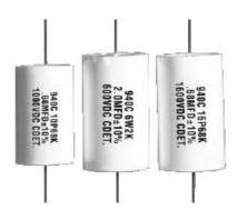
Type 940C round, axial film capacitors use polypropylene film and dual metallized electrodes for both self healing properties and high peak current carrying capability (dV/dt). This series features low ESR characteristics, excellent high frequency and high voltage capabilities.
