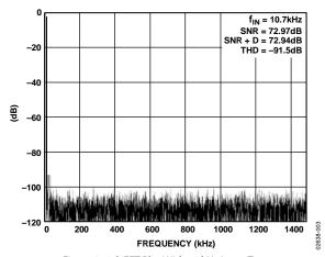
Figure 3. 64k FFT Plot With 10 kHz Input Tone
