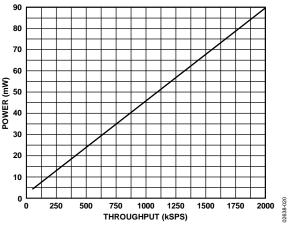
Figure 20. Nap Mode, Power vs. Throughput
