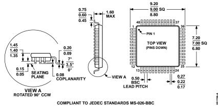
Figure 33. 48-Lead Plastic Quad Flatpack [LQFP] (ST-48) Dimensions shown in millimeters
