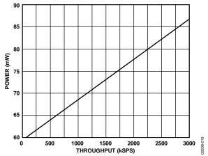
Figure 19. Normal Mode, Power vs. Throughput
