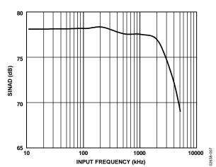
Figure 7. SINAD vs. Input Tone (AD8021 Input Circuit)
