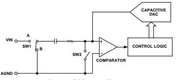
Figure 12. ADC Conversion Phase
