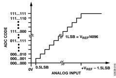
Figure 16. AD7482 Transfer Characteristic
