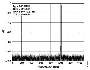
Figure 4. 64k FFT Plot With 1 MHz Input Tone
