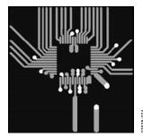
Figure 24. Top Layer Routing
