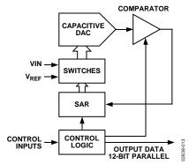
Figure 11. Simplified Block Diagram of the AD7482
