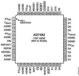
Figure 2. Pin Configuration
