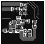
Figure 28. Silkscreen and Bottom Layer Routing
