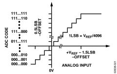
Figure 21. Transfer Characteristic with Positive Offset
