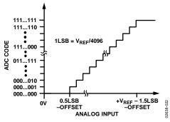
Figure 22. Transfer Characteristic with Negative Offset
