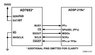
Figure 37. Interfacing the AD7653 to an SPI Interface
