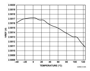
Figure 17. Typical Reference Output Voltage vs. Temperature
