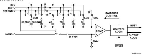
Figure 20. ADC Simplified Schematic
