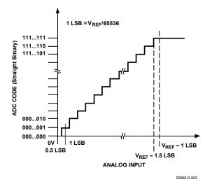
Figure 21. ADC Ideal Transfer Function
