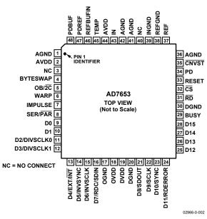
Figure 4. 48-Lead LQFP (ST-48) and 48-Lead LFCSP (CP-48)
