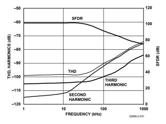
Figure 11. THD, Harmonics, and SFDR vs. Frequency
