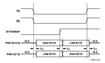
Figure 31. 8-Bit Parallel Interface
