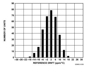
Figure 18. Reference Voltage Temperature Coefficient Distribution (335 Units)
