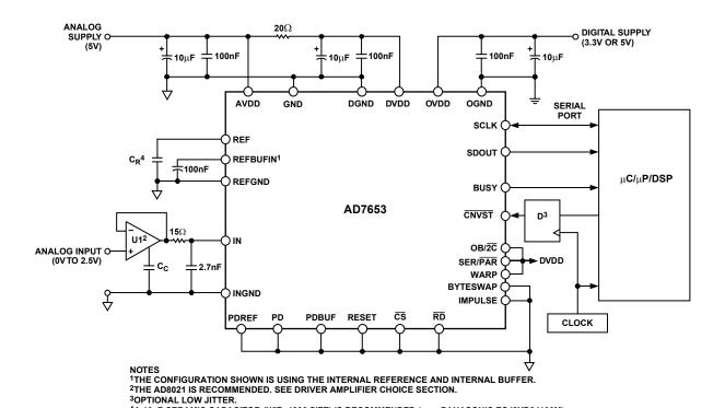
4A 10,1F CERAMIC CAPACITOR (X5R, 1206 SIZE) IS RECOMMENDED (e.g., PANASONIC ECJ3YB0J106M). SEE VOLTAGE REFERENCE INPUT SECTION.
