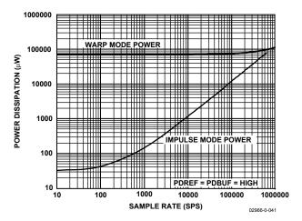
Figure 25. Power Dissipation vs. Sampling Rate
