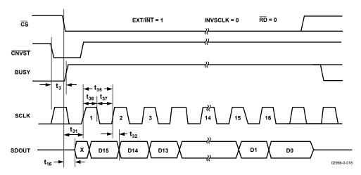
Figure 35. Slave Serial Data Timing for Reading (Read Previous Conversion during Convert)
