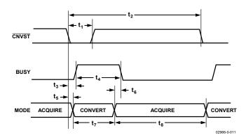
Figure 26. Basic Conversion Timing
