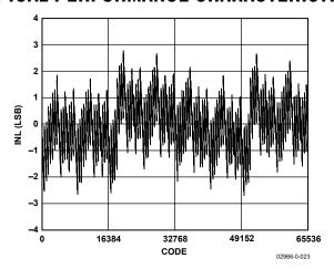
Figure 5. Integral Nonlinearity vs. Code
