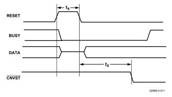
Figure 27. RESET Timing
