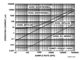
Figure 15. Operating Current vs. Sample Rate
