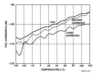
Figure 14. THD and Harmonics vs. Temperature
