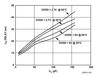
Figure 19. Typical Delay vs. Load Capacitance C<sub>L</sub>
