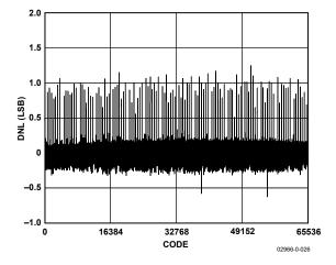
Figure 8. Differential Nonlinearity vs. Code
