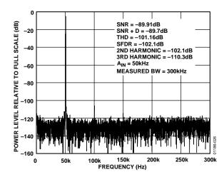
Figure 26. 16 K Point FFT (Output Data Rate = 600 kHz)
