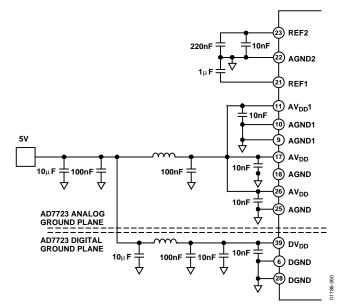
Figure 50. Reference and Power Supply Decoupling
