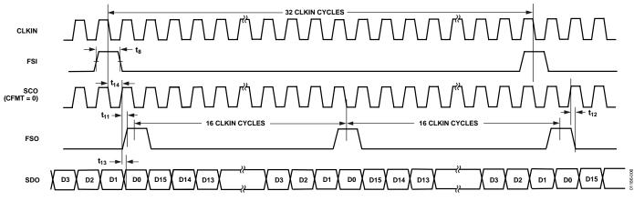
Figure 6. Serial Mode 3: Timing for Frame Sync Input, Frame Sync Output, Serial Clock Output, and Serial Data Output (See Table 3 for Control Inputs, TSI = DOE)
