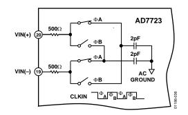
Figure 36. Analog Input Equivalent Circuit
