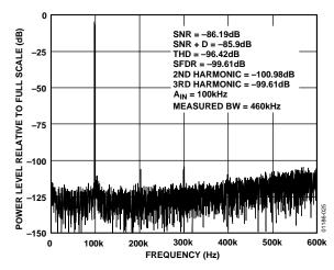
Figure 25. 16 K Point FFT (Output Data Rate = 1.2 MHz)
