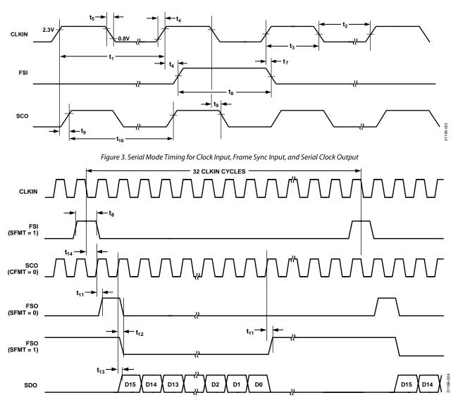
Figure 4. Serial Mode 1: Timing for Frame Sync Input, Frame Sync Output, Serial Clock Output, and Serial Data Output (See Table 3 for Control Inputs, TSI = DOE)
