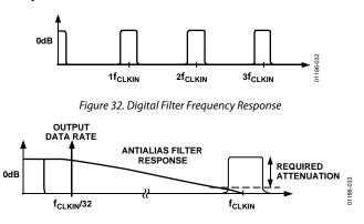
Figure 33. Frequency Response of Antialias Filter
