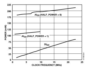
Figure 24. Power Consumption vs. CLKIN Frequency
