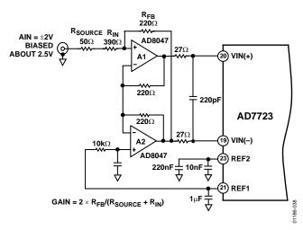
Figure 38. Single-Ended-to-Differential Input Circuit for Bipolar Mode Operation (Analog Input Biased About 2.5 V)
