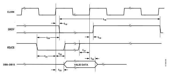
Figure 9. Parallel Mode Read Timing,  $\overline{CS} = \overline{RD}$
