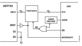
Figure 44. Parallel Interface Connection
