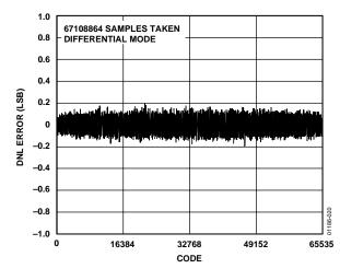
Figure 20. Differential Nonlinearity (Output Data Rate = 1.2 MHz)
