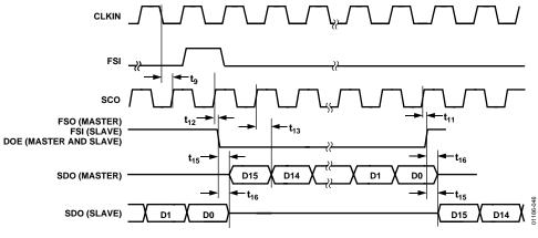
Figure 46. Serial Mode 1 Timing for Two-Channel Multiplexed Operation
