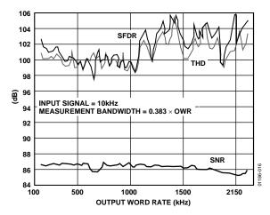
Figure 16. SNR, THD, and SFDR vs. Sampling Frequency (Decimate by 16)
