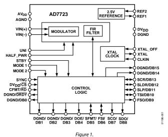
The part provides an on-chip 2.5 V reference. Alternatively, an external reference can be used.
