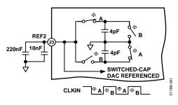
Figure 41. REF2 Equivalent Input Circuit
