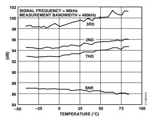
Figure 14. SNR and THD vs. Temperature (Output Data Rate = 1.2 MHz)
