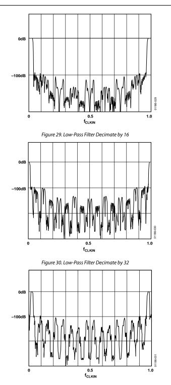
Figure 31. Band-Pass Filter Decimate by 32
