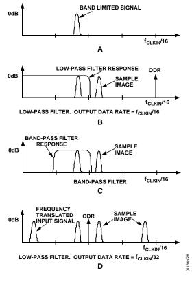
Figure 28. Band-Pass Operation
