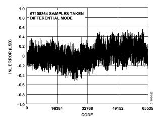
Figure 22. Integral Nonlinearity (Output Data Rate = 1.2 MHz)
