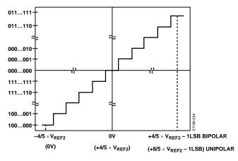
Figure 34. Bipolar (Unipolar) Mode Transfer Function
