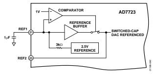
Figure 40. Reference Circuit Block Diagram
