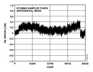
Figure 23. Integral Nonlinearity (Output Data Rate = 600 kHz)
