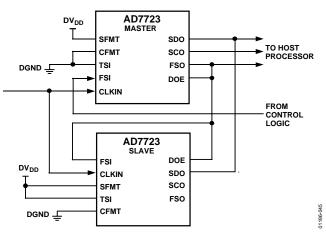
Figure 45. Serial Mode 1 Connection for Two-Channel Multiplexed Operation
