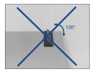
3 Rotate down the actuator until firmly closed. It is critical that the inserted FPC is not moved and remains fully inserted.
