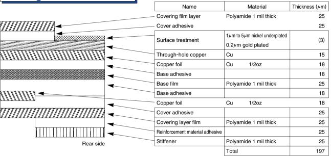
To prevent release of the lock due to FPC bending, use of the FPC with copper foil on rear side is NOT RECOMMENDED.
