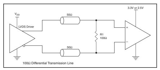
Figure 4. Typical LVDS Driver Termination
