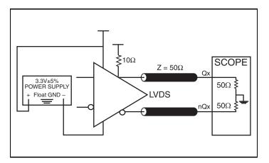
3.3V Output Load AC Test Circuit
