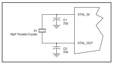
Figure 2. Crystal Input Interface
