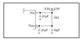
Figure 1. Power Supply Filtering
