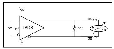
**Differential Offset Voltage Setup**
