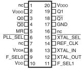
ICS844002-01 20-Lead TSSOP 6.5mm x 4.4mm x 0.925mm package body G Package Top View
