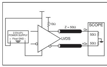
2.5V Output Load AC Test Circuit
