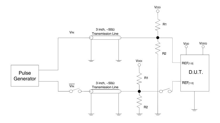
Test Circuit for Differential Input<sup>(1)</sup>
