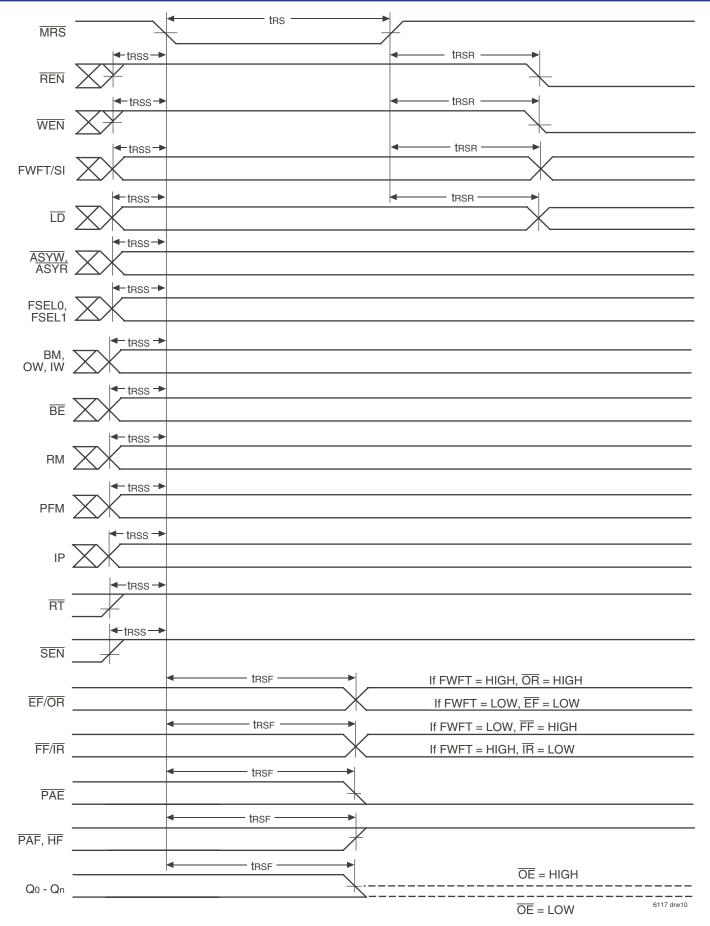
Figure 5. Master Reset Timing
