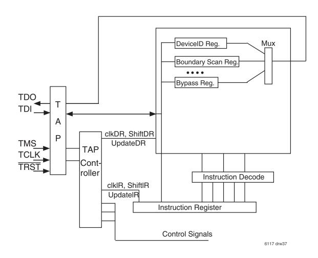
Figure 32. Boundary Scan Architecture
