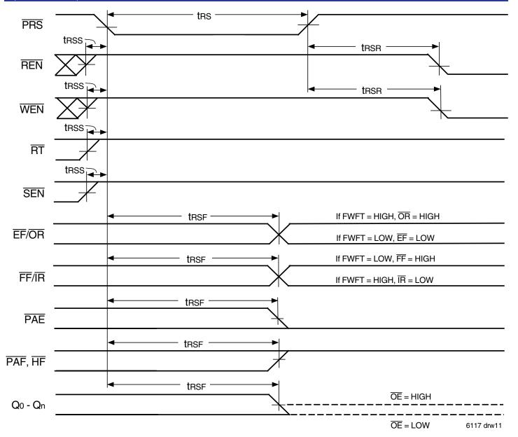
Figure 6. Partial Reset Timing
