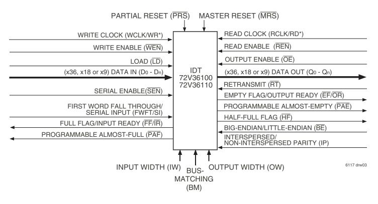
Figure 1. Single Device Configuration Signal Flow Diagram
