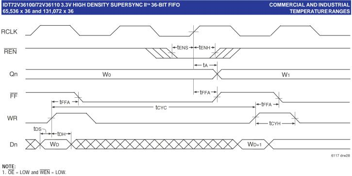
Figure 23. Asynchronous Write, Synchronous Read, Full Flag Operation (IDT Standard Mode)
