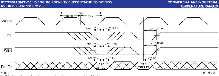
1. This timing diagram illustrates programming with an input bus width of 36 bits.
