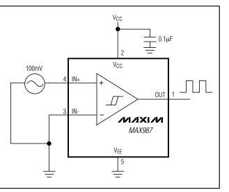
Figure 3. Zero-Crossing Detector
