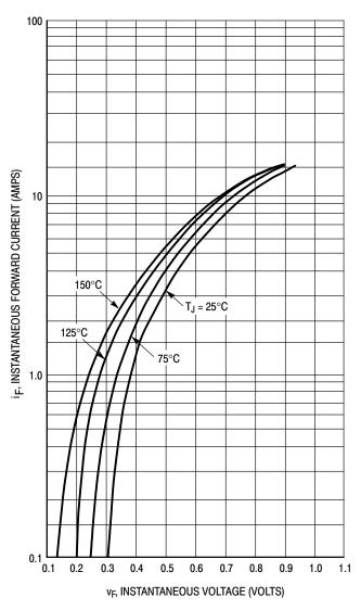
Figure 1. Typical Forward Voltage
