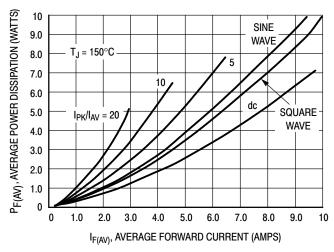
Figure 3. Average Power Dissipation
