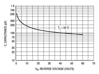
Figure 6. Typical Capacitance
