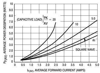
Figure 3. Power Dissipation
