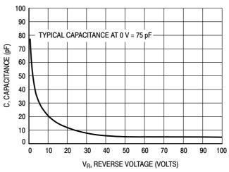
Figure 10. Typical Capacitance
