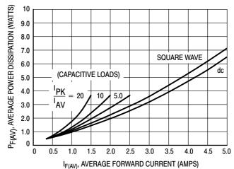
Figure 8. Power Dissipation
