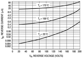
Figure 2. Typical Reverse Current\*
