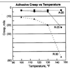
3M Test Method – Inclined Plane Static Shear Test Method;  $30^{\circ}$  incline, tested on ABS using ½ inch diameter die cuts from SJ-5816, SJ-6016 and SJ-6216 Rollstock products. 2 lb. Load per ½ inch diameter die cut. Measured time of creep: 15 minutes.
