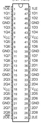
These devices can be used as two 8-bit latches or one 16-bit latch. When the latch-enable (LE) input is high, the Q outputs follow the data (D) inputs. When LE is taken low, the Q outputs are latched at the levels at the D inputs.
