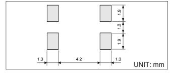
Remarks 1. Do not connect terminals #2, #3 to external device and GND. These are dummy terminals.
