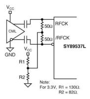
Figure 11d. CML Interface (AC-Coupled)
