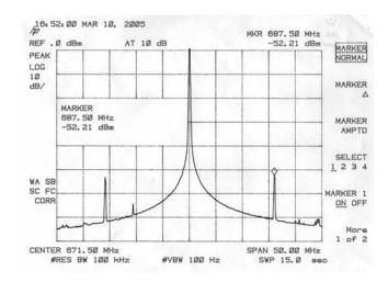
Figure 4b. Reference Spur at -52dB at 16MHz (R =  $130\Omega$ , C1 =  $0.47\mu$ F, C2 = 1000pF)
