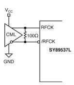
Figure 11c. CML Interface (DC-Coupled)
