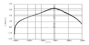
Figure 9. VCO Gain vs. Loop Filter Control Voltage at 3.3V,  $T_A = 25$ °C
