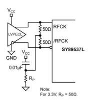
Figure 11a. LVPECL Interface (DC-Coupled)
