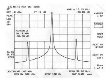
Figure 4a. Reference Spur at -39dB at 16MHz  $(R = 130\Omega, C1 = 0.47\mu F, C2 = 100pF)$
