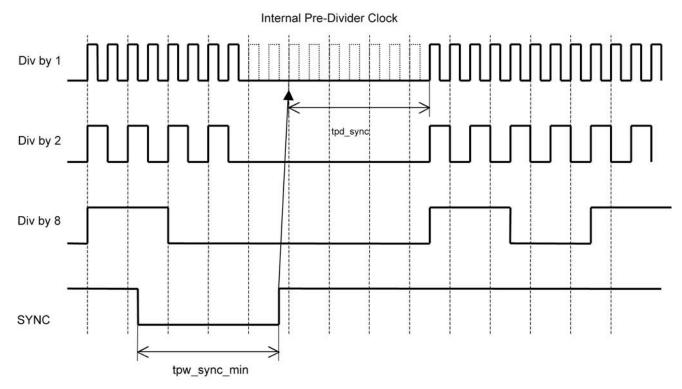
**Output Synchronization Controlled by SYNC Timing Diagram**
