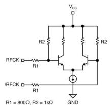
Figure 10. Simplified Input Structure
