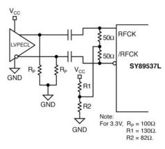
Figure 11b. LVPECL Interface (AC-Coupled)
