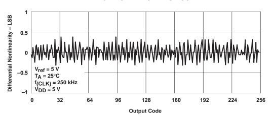
Figure 11. Differential Nonlinearity With Output Code
