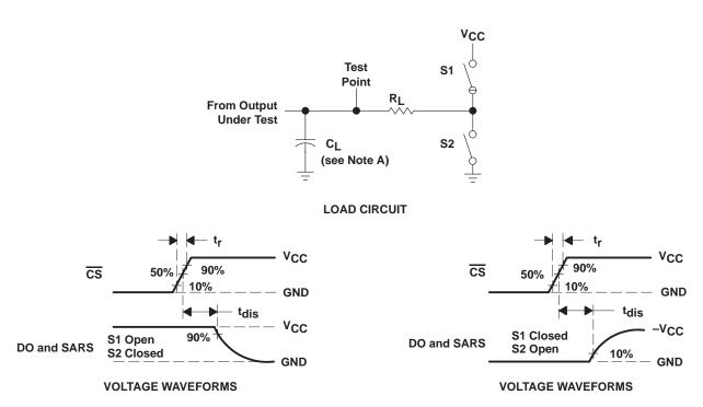
NOTE A: C<sub>I</sub> includes probe and jig capacitance.
