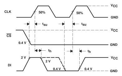
Figure 1. Data-Input Timing
