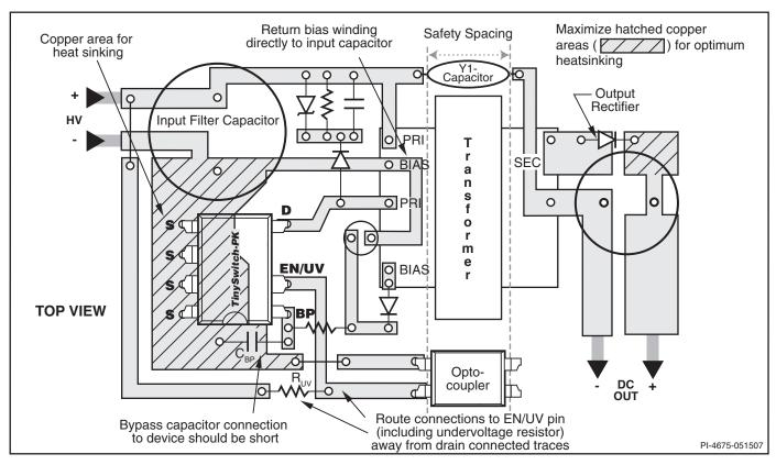
Figure 16. Layout Considerations for TinySwitch-PK Using P Package.
