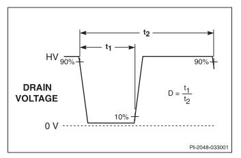
Figure 18. Duty Cycle Measurement.
