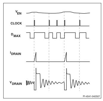
Figure 9. Operation at Very Light Load ( $f_{\rm osc}$  132 kHz).
