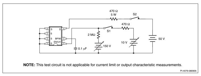
Figure 17. General Test Circuit.
