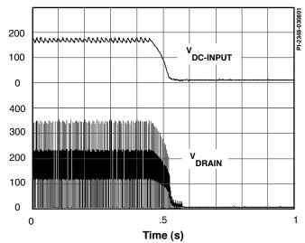
Figure 12. Normal Power-down Timing (Without UV Resistor).
