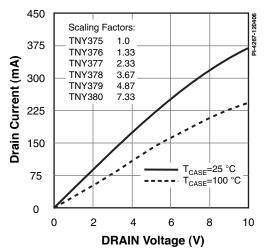
Figure 25. Output Characteristics.
