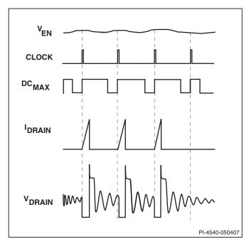
Figure 8. Operation at Medium Loading (fosc 132 kHz).
