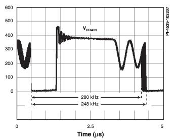
Figure 4. Frequency Jitter.
