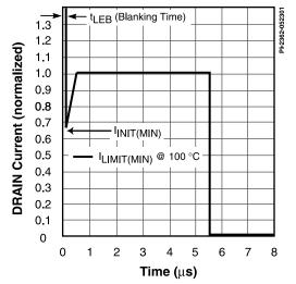
Figure 20. Current Limit Envelope at  $f_{\rm OSC}$  = 132 kHz.
