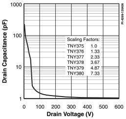
Figure 26.  $C_{\rm oss}$  vs. Drain Voltage.
