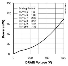
Figure 27. Drain Capacitance Power.
