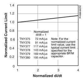
Figure 24. Current Limit vs. di/dt.
