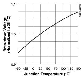
Figure 21. Breakdown vs. Temperature.
