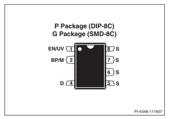
Figure 3. Pin Configuration.
