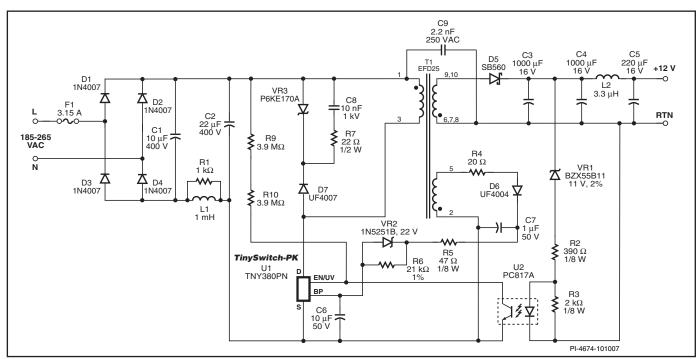
Figure 15. Single 230 VAC Input 20 W Continuous and 45 W Peak Power Supply Using TNY380PN.
