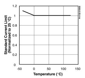
Figure 23. Standard Current Limit vs. Temperature.
