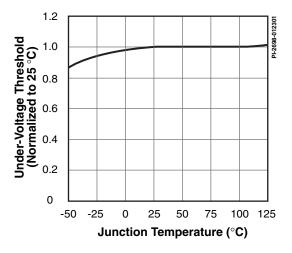
Figure 28. Undervoltage Threshold vs. Temperature.
