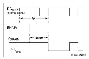
Figure 19. Output Enable Timing.
