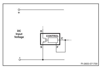
Figure 15. Half Frequency Operation (66 kHz).
