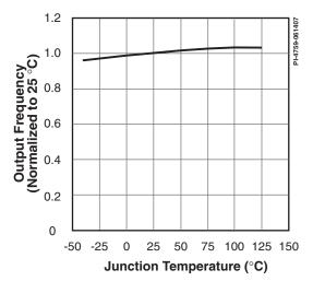
Figure 57. Frequency vs. Temperature.
