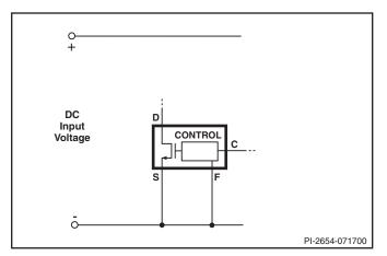
Figure 14. Full Frequency Operation (132 kHz).
