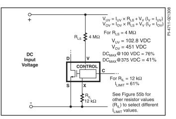
Figure 5. TOP254-258 Y and All M/E/L Package Line Sense and Externally Set Current Limit.
