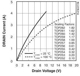
Figure 66. Output Characteristics.
