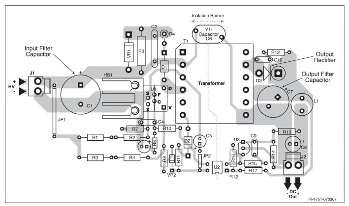
Figure 48. Layout Considerations for TOPSwitch-HX Using TOP254-258 Y-Package.
