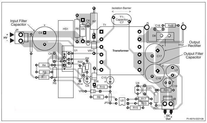
Figure 50a. Layout Considerations for TOPSwitch-HX Using E-Package and Operating at 66 kHz.
