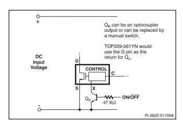
Figure 24. Active-on (Fail Safe) Remote ON/OFF.
