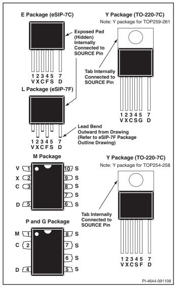
Figure 4. Pin Configuration (Top View).
