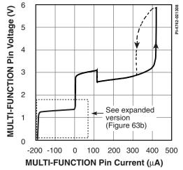
Figure 63a. MULTI-FUNCTION Pin Voltage vs. Current.
