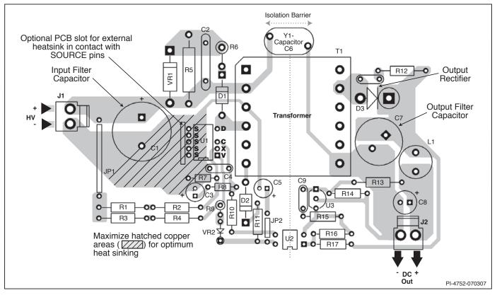
Figure 47. Layout Considerations for TOPSwitch-HX Using M-Package.
