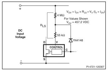
Figure 21. Line-Sensing for Overvoltage Only (Undervoltage Disabled). Maximum Duty Cycle Reduced at Low Line and Further Reduction with Increasing Line Voltage.
