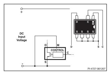
Figure 29. Three Terminal Operation (MULTI-FUNCTION Features Disabled).
