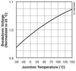
Figure 56. Breakdown Voltage vs. Temperature.
