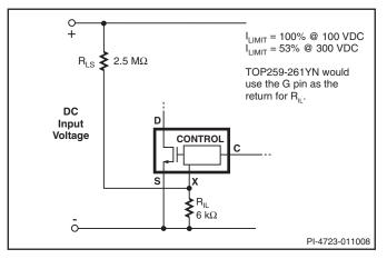
Figure 23. Current Limit Reduction with Line Voltage.
