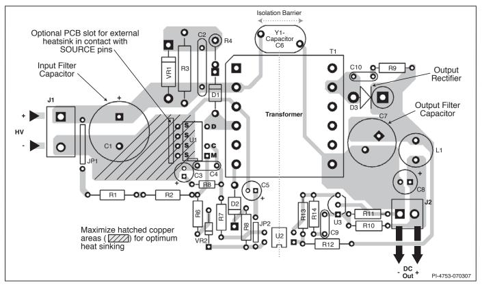
Figure 46. Layout Considerations for TOPSwitch-HX Using P-Package.
