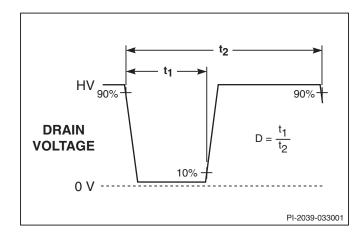
Figure 51. Duty Cycle Measurement.
