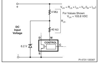
Figure 33. Line Sensing for Undervoltage Only (Overvoltage Disabled).
