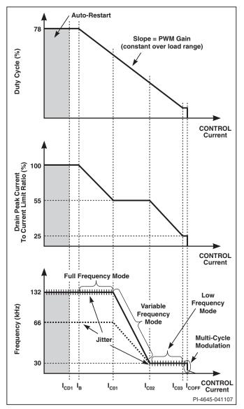
Figure 9. Control Pin Characteristics (Multi-Mode Operation).
