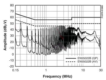
Figure 45a. Fixed Frequency Operation Without Jitter.
