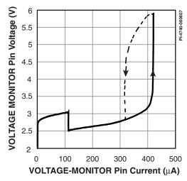
Figure 62a. VOLTAGE-MONITOR Pin vs. Current.
