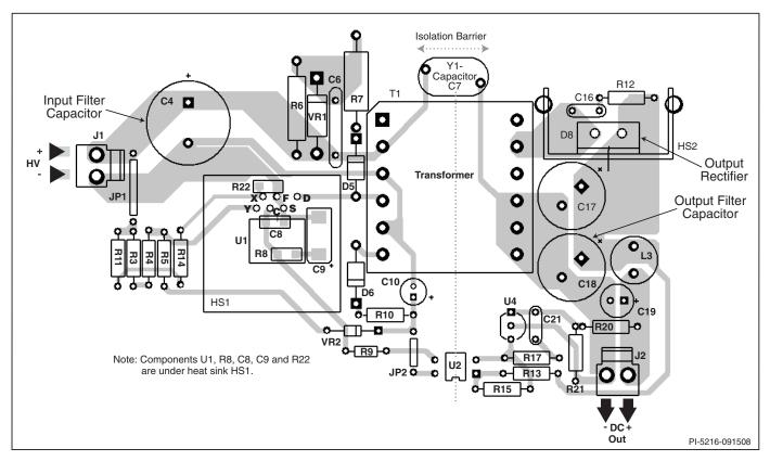
Figure 50c. Layout Considerations for TOPSwitch-HX Using L-Package and Operating at 132 kHz.
