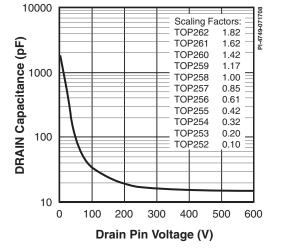
Figure 68. C<sub>oss</sub> vs. DRAIN Voltage.
