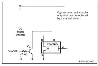
Figure 37. Active-on (Fail Safe) Remote ON/OFF.
