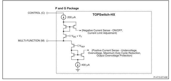
Figure 13b. MULTI-FUNCTION (M) Pin Input Simplified Schematic.
