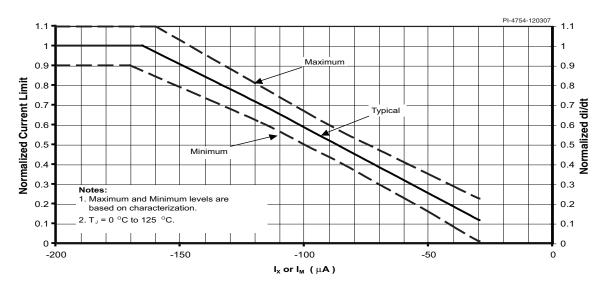
Figure 55a. Normalized Current Limit vs. X or M Pin Current.
