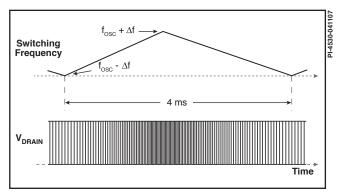
Figure 10. Switching Frequency Jitter (Idealized V<sub>DRAIN</sub> Waveforms).
