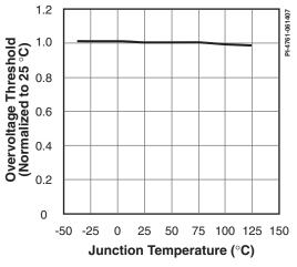
Figure 60. Overvoltage Threshold vs. Temperature.
