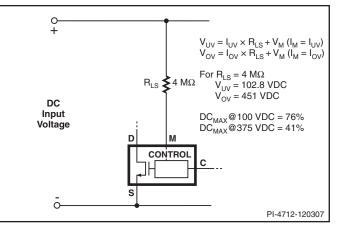
Figure 7. P/G Package Line Sense.
