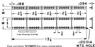
Five sections **SCORED** for easy separation. M'tg. Holes in each section.
