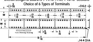
Five sections **SCORED** for easy separation. M'tg. Holes in each section.
