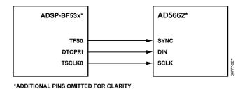
Figure 37. AD5662 to Blackfin ADSP-BF53x Interface
