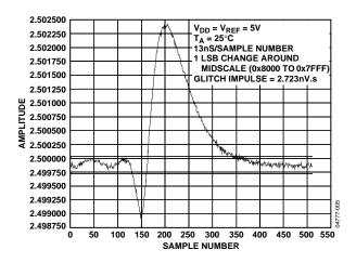
Figure 25. Digital-to-Analog Glitch Impulse (Negative)
