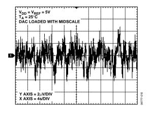
Figure 30. 0.1 Hz to 10 Hz Output Noise Plot
