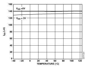
Figure 17. Supply Current vs. Temperature
