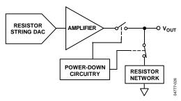
Figure 36. Output Stage During Power-Down
