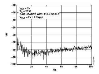
Figure 28. Total Harmonic Distortion
