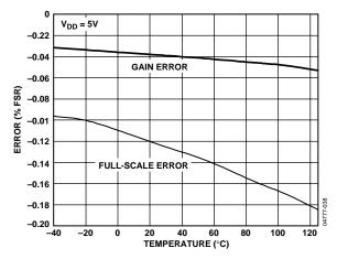
Figure 10. Gain Error and Full-Scale Error vs. Temperature
