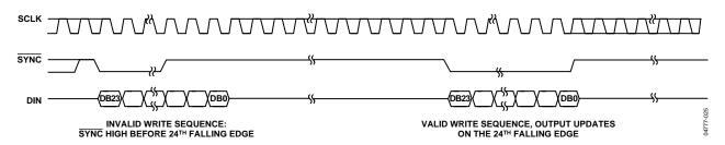
Figure 35. SYNC Interrupt Facility
