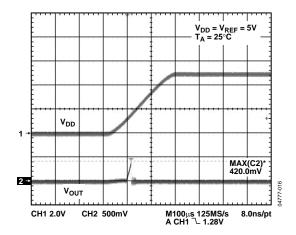
Figure 22. Power-On Reset to 0 V
