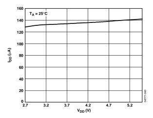
Figure 18. Supply Current vs. Supply Voltage
