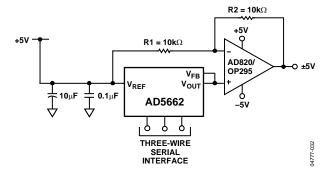
Figure 42. Bipolar Operation with the AD5662
