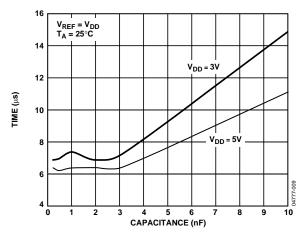
Figure 29. Settling Time vs. Capacitive Load
