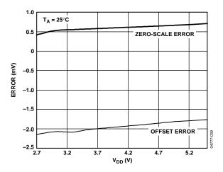
Figure 13. Zero-Scale and Offset Error vs. Supply
