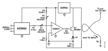
Figure 43. Programmable 4-20 mA Process Controller
