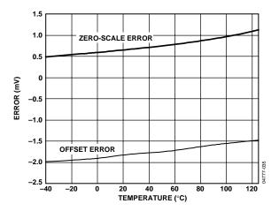
Figure 11. Zero-Scale and Offset Error vs. Temperature
