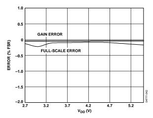
Figure 12. Gain Error and Full-Scale Error vs. Supply
