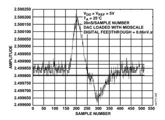
Figure 27. Digital Feedthrough
