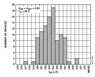
Figure 14.  $I_{DD}$  Histogram with  $V_{DD} = 5.5 V$
