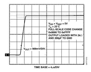
Figure 21. Full-Scale Settling Time, 5 V
