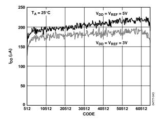
Figure 16. Supply Current vs. Code
