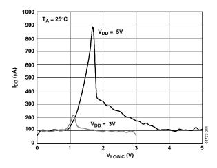
Figure 19. Supply Current vs. Logic Input Voltage
