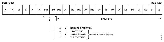
Figure 34. Input Register Contents
