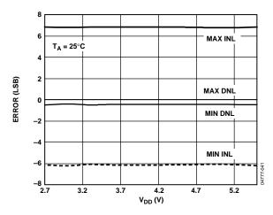
Figure 9. INL and DNL Error vs. Supply
