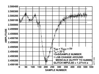
Figure 26. Digital-to-Analog Glitch Impulse (Positive)
