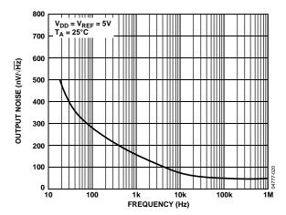
Figure 31. Noise Spectral Density
