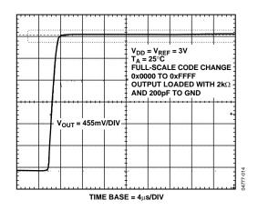
Figure 20. Full-Scale Settling Time, 3 V
