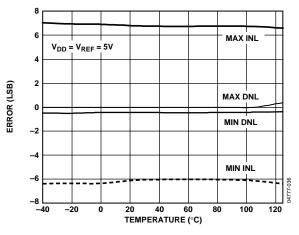
Figure 7. INL Error and DNL Error vs. Temperature
