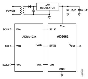
Figure 44. AD5662 with a Galvanically Isolated Interface
