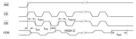
Notes: 1. Toggling either  $\overline{OE}$  or  $\overline{CE}$  or both  $\overline{OE}$  and  $\overline{CE}$  will operate toggle bit. The t<sub>OEHP</sub> specification must be met by the toggling input(s).
