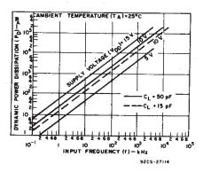
Fig. 10 — Typical dynamic power dissipation vs. frequency.
