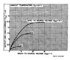
Fig.2 — Minimum output low (sink) current characteristics.
