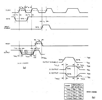
Fig.5 — Functional waveforms for CD4076B.
