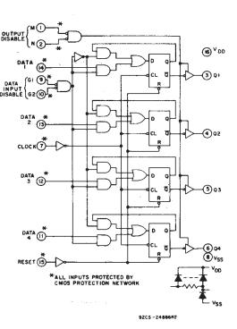
Fig.8 - CD4076B logic diagram.
