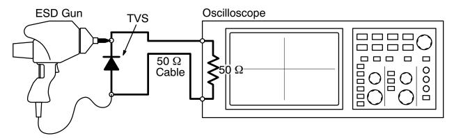
Figure 4. Diagram of ESD Test Setup
