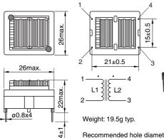
Recommended hole diameter: ø1.3 Dimensions in mm
