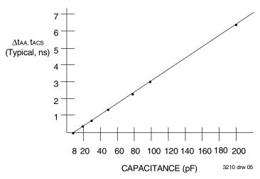
Figure 3. Output Capacitive Derating
