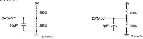
\*Including jig and scope capacitance.
