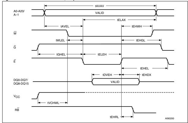
Figure 11. Write AC Waveforms, Chip Enable Controlled
