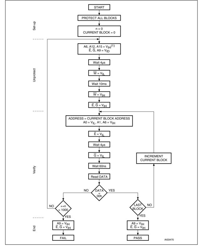
Figure 17. Programmer Equipment Chip Unprotect Flowchart
