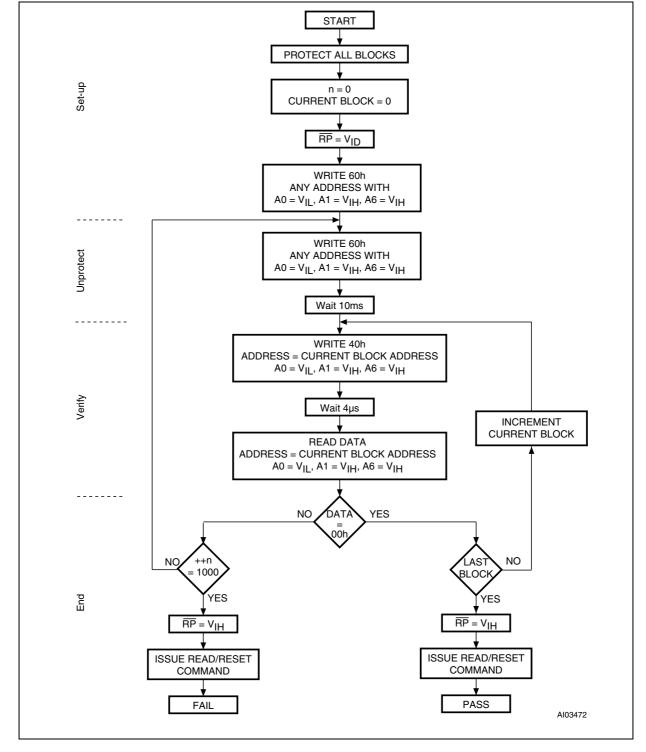
Figure 19. In-System Equipment Chip Unprotect Flowchart
