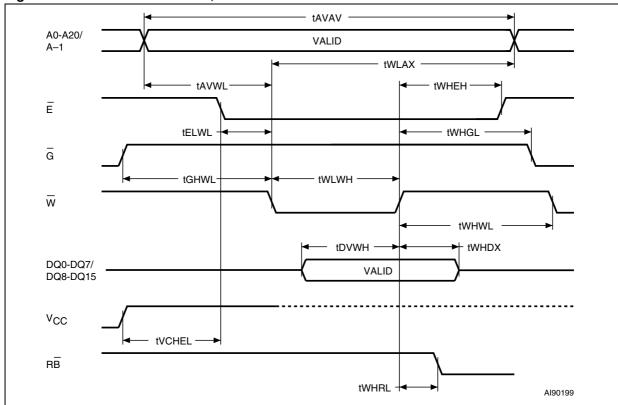
Figure 10. Write AC Waveforms, Write Enable Controlled
