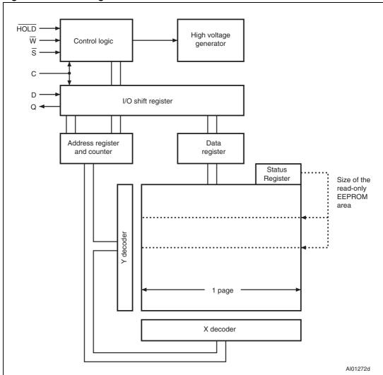
Figure 6. Block diagram
