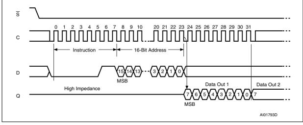
1. Depending on the memory size, as shown in *Table 7*., the most significant address bits are Don't Care.
