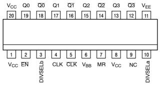
NOTE: All  $V_{CC}$  pins are tied together on the die. Warning: All  $V_{\mbox{\footnotesize CC}}$  and  $V_{\mbox{\footnotesize EE}}$  pins must be externally connected to Power Supply to guarantee proper operation.
