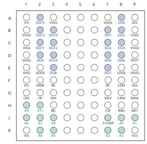
Notes: 1.D9 should be connected to Vss or VssQ in normal operations.
