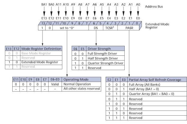
Notes: 1. On-chip temperature sensor is used in place of TCSR. Setting these bits will have no effect.
