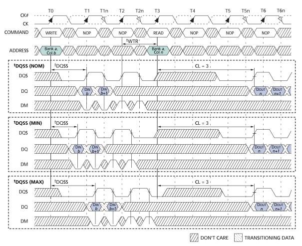
Notes: 1. DIN b = data-in for column b; DOUT n = data-out for column n.
