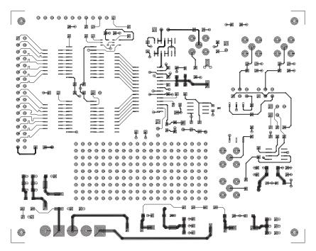
Figure 30. Board Layout, Layer 1
