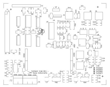
Figure 34. Board Layout, Layer 5
