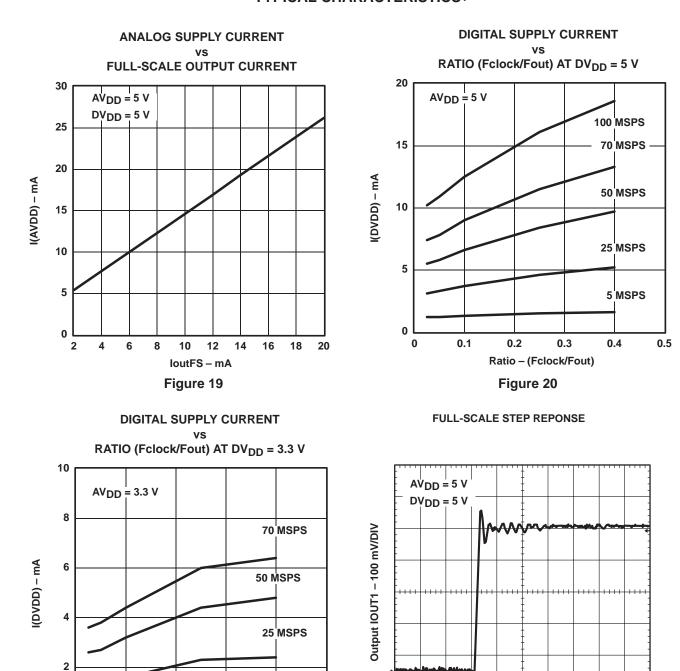
$^\dagger$  AV<sub>DD</sub> and DV<sub>DD</sub> specified for each chart seperately, IOUT<sub>FS</sub> = 20 mA, single-ended output IOUT1, 50  $\Omega$  doubly terminated load, T<sub>A</sub> = 25°C (unless otherwise noted.)
