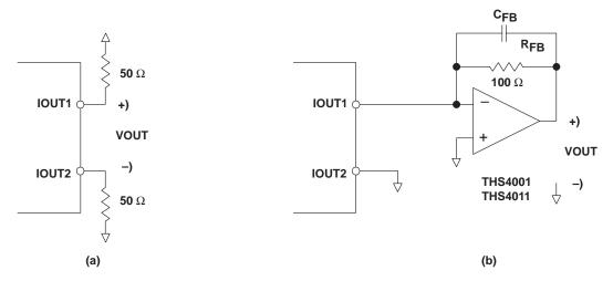
Figure 27. Differential and Single-Ended Output Configuration
