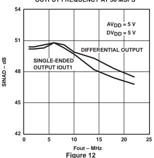
$<sup>^\</sup>dagger$  AV<sub>DD</sub> and DV<sub>DD</sub> specified for each chart seperately, IOUT<sub>FS</sub> = 20 mA, single-ended output IOUT1, 50  $\Omega$  doubly terminated load, T<sub>A</sub> = 25°C (unless otherwise noted.)
