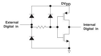
Figure 24. Digital Equivalent Input
