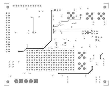
Figure 33. Board Layout, Layer 4
