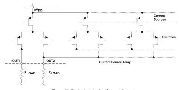
Figure 26. Equivalent Analog Current Output
