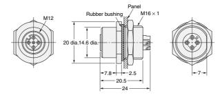
XS2P-D422-1 (with DIP Pins) XS2P-D422-2 (with Solder Cup Pins) Front Lock Model
