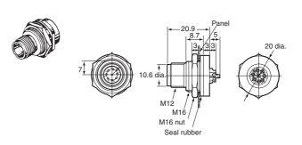
XS2P-D822-2 Panel-mounting Socket (M12) with Solder Cup Pins and Front Lock
