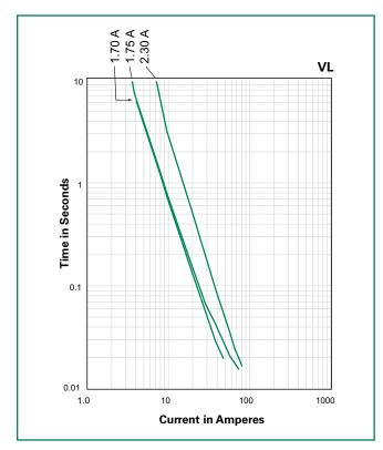
The average time current curves and Temperature Rerating curve performance is affected by a number or variables, and these curves provided as guidance only. Customer must verify the performance in their application.
