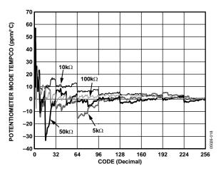
Figure 19. Potentiometer Mode Tempco  $(\Delta V_W x 10^6)/(V_W x \Delta T)$  vs. Code
