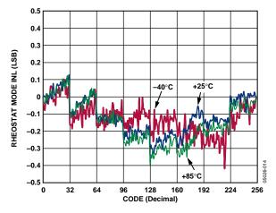
Figure 12. R-INL vs. Code vs. Temperature
