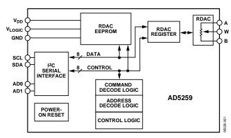
Figure 1. Block Diagram
