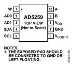
Figure 5. Pin Configuration
