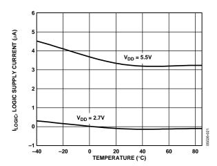
Figure 17. Logic Supply Current vs. Temperature vs. V<sub>DD</sub>
