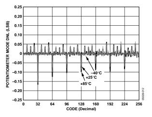
Figure 9. DNL vs. Code vs. Temperature
