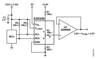
Figure 46. V<sub>COM</sub> Adjustment Application
