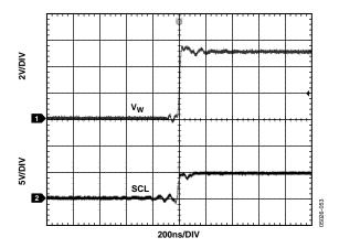
Figure 31. Large Signal Settling Time
