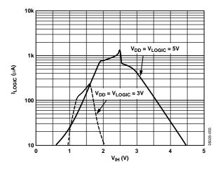
Figure 27. Logic Supply Current vs. Input Voltage
