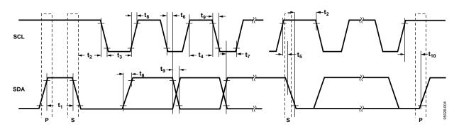
Figure 4. I<sup>2</sup>C Interface Timing Diagram
