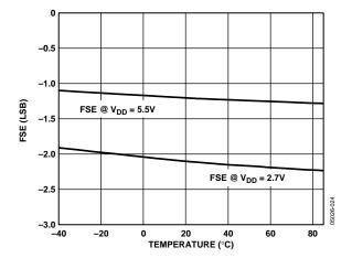
Figure 14. Full-Scale Error vs. Temperature
