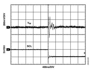
Figure 29. Digital Feedthrough
