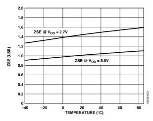
Figure 15. Zero-Scale Error vs. Temperature
