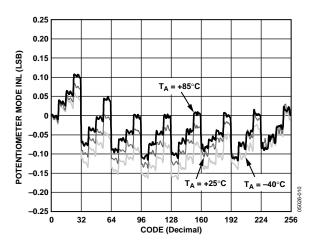
Figure 8. INL vs. Code vs. Temperature
