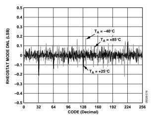
Figure 13. R-DNL vs. Code vs. Temperature
