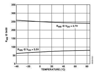
Figure 20. R<sub>WB</sub> vs. Temperature
