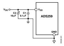
Figure 44. Power Supply Bypassing
