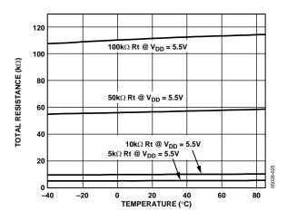
Figure 21. Total Resistance vs. Temperature
