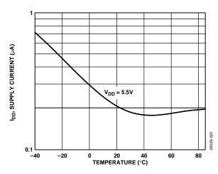
Figure 16. Supply Current vs. Temperature
