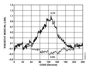
Figure 6. R-INL vs. Code vs. Supply Voltage
