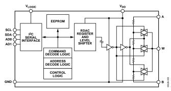
Figure 2. Block Diagram Showing Level Shifters
