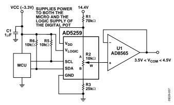
Figure 47. Circuitry When a Separate Supply is Not Available for  $V_{DD}$
