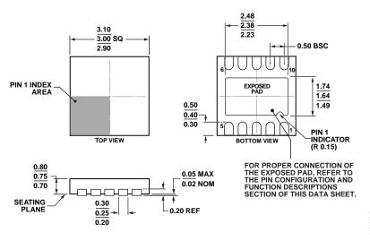
Figure 49. 10-Lead Lead Frame Chip Scale Package [LFCSP\_WD] 3 mm × 3 mm Body, Very Very Thin, Dual Lead (CP-10-9) Dimensions shown in millimeters
