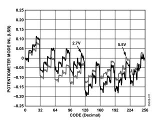
Figure 10. INL vs. Supply Voltages
