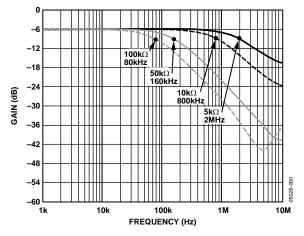
Figure 26. -3 dB Bandwidth @ Code =  $0 \times 80$
