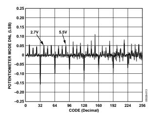
Figure 11. DNL vs. Code vs. Supply Voltage
