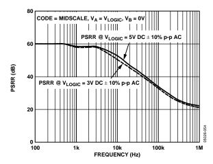
Figure 28. PSRR vs. Frequency
