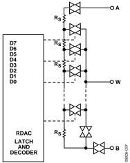
Figure 39. AD5259 Equivalent RDAC Circuit
