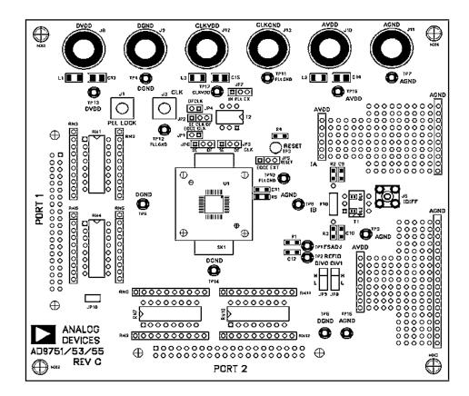
Figure 36. Evaluation Board, Assembly-Top
