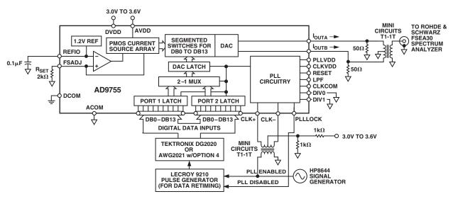
Figure 2. Basic AC Characterization Test Setup
