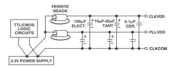
Figure 9. LC Network for Power Filtering
