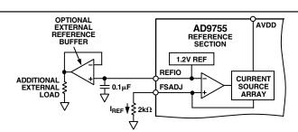
Figure 4. Internal Reference Configuration
