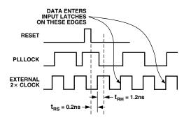
Figure 12. Reset Function Timing with PLL Disabled
