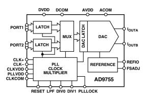
The DAC utilizes a segmented current source architecture combined with a proprietary switching technique to reduce glitch energy and maximize dynamic accuracy. Differential current outputs support single-ended or differential applications. The differential outputs each provide a nominal full-scale current from 2 mA to 20 mA.
