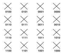
Figure 27. 16 QAM Constellation, Gray Coded (Two 4-Level PAM Signals with Orthogonal Carriers)
