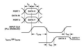
Figure 1. I/O Timing
