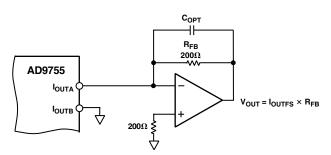
Figure 24. Unipolar Buffered Voltage Output
