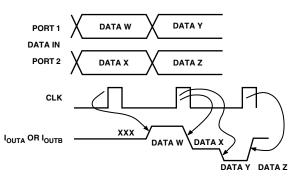
Figure 7b. DAC Input Timing Requirements with PLL Active, Multiple Clock Cycles
