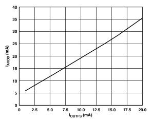
Figure 17. I<sub>AVDD</sub> vs. I<sub>OUTFS</sub>
