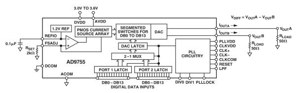
Figure 3. Simplified Block Diagram
