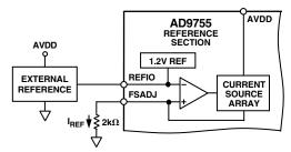
Figure 5. External Reference Configuration
