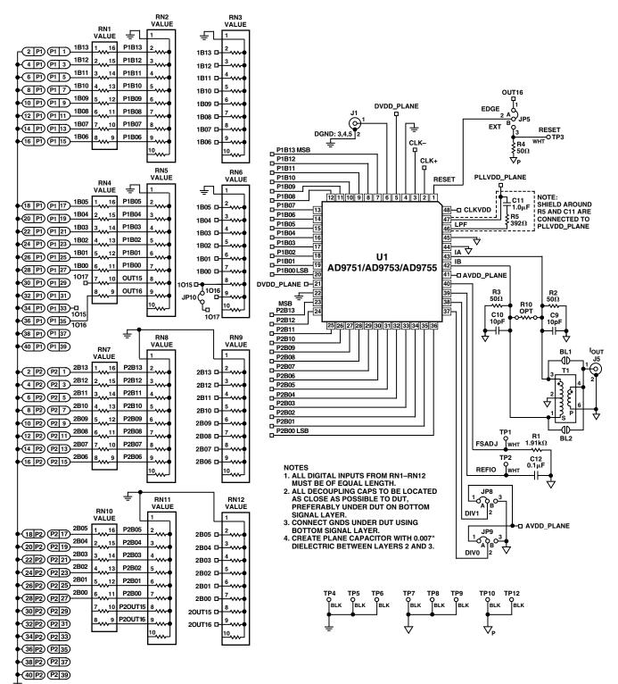
Figure 34. Evaluation Board Circuitry
