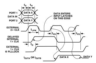
Figure 11. Timing Requirements, Interleaved (2×) Mode with PLL Disabled
