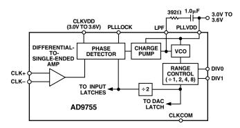
Figure 6. Clock Circuitry with PLL Active
