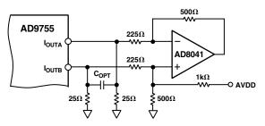
Figure 22. Single-Supply DC Differential Coupled Circuit
