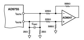
Figure 21. DC Differential Coupling Using an Op Amp
