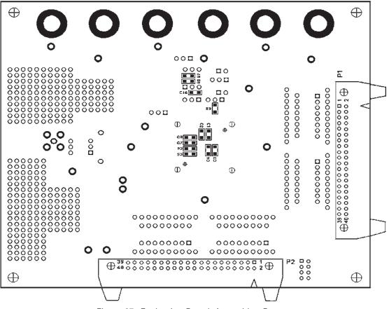
Figure 37. Evaluation Board, Assembly-Bottom
