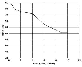
Figure 25. Power Supply Rejection Ratio
