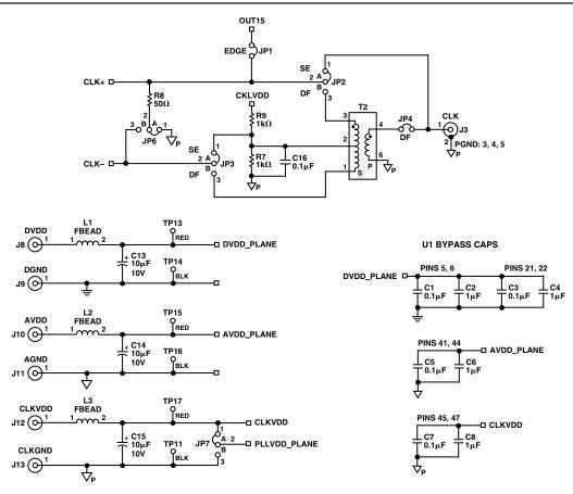
Figure 35. Evaluation Board Clock Circuitry
