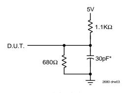
or equivalent circuit Figure 1. Output Load \*Includes jig and scope capacitances.
