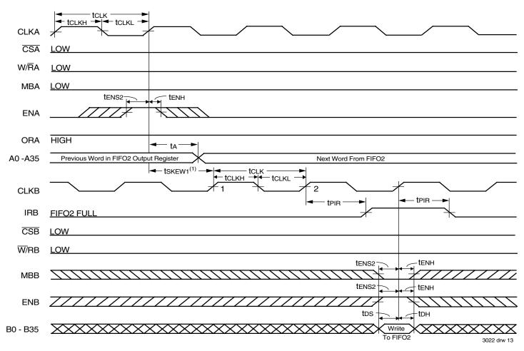
1. tskew1 is the minimum time between a rising CLKA edge and a rising CLKB edge for IRB to transition HIGH in the next CLKB cycle. If the time between the rising CLKA edge and rising CLKB edge is less than tskew1, then IRB may transition HIGH one CLKB cycle later than shown.
