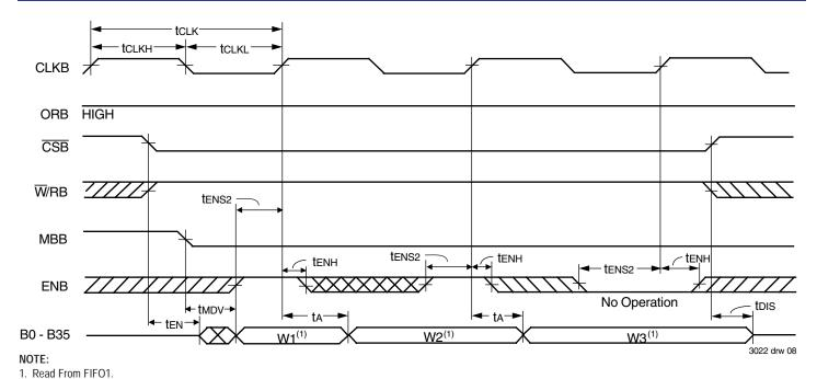
Figure 6. Port B Read Cycle Timing for FIFO1
