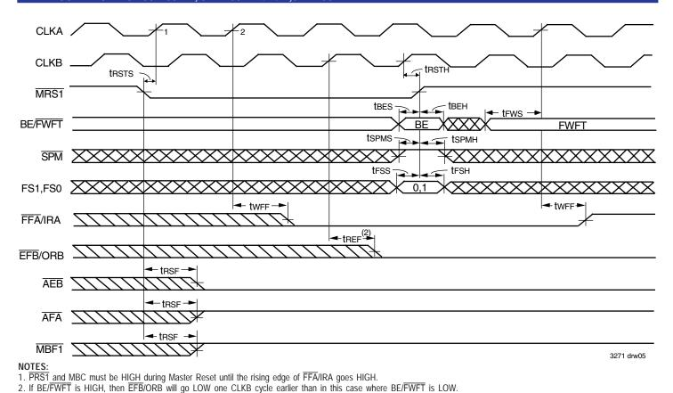
Figure 4. FIFO1 Master Reset and Loading X1 and Y1 with a Preset Value of Eight (IDT Standard and FWFT Modes)
