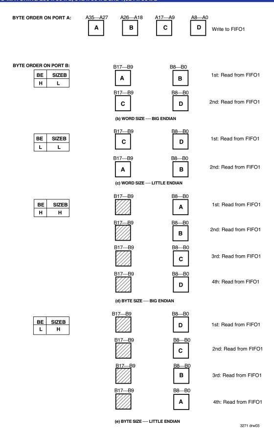
Figure 3. Port C Bus Sizing
