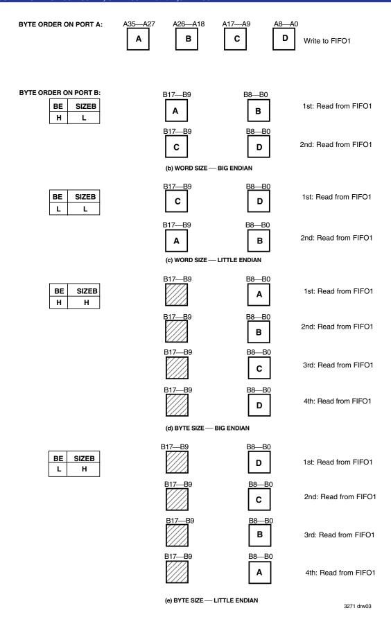
Figure 2. Port B Bus Sizing
