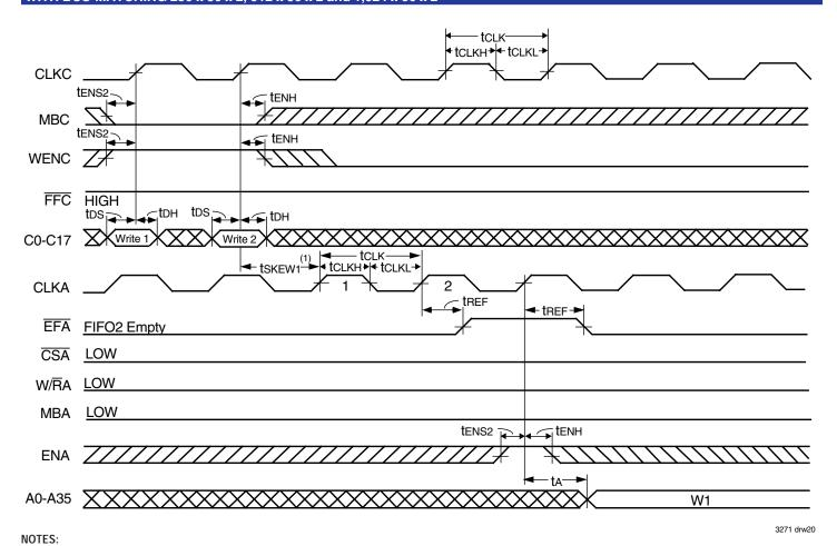
1. tskew1 is the minimum time between a rising CLKC edge and a rising CLKA edge for EFA to transition HIGH in the next CLKA cycle. If the time between the rising CLKC edge and rising CLKA edge is less than tskew1, then the transition of EFA HIGH may occur one CLKA cycle later than shown.
