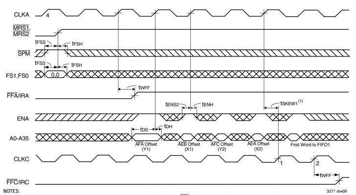
1. tskew1 is the minimum time between the rising CLKA edge and a rising CLKC edge for FFC/IRC to transition HIGH in the next cycle. If the time between the rising edge of CLKA and rising edge of CLKC is less than tskewi, then FFC/IRC may transition HIGH one CLKC cycle later than shown.
