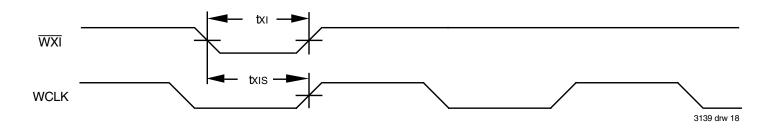
Figure 18. Write Expansion In Timing
