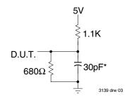
Figure 1. Output Load
