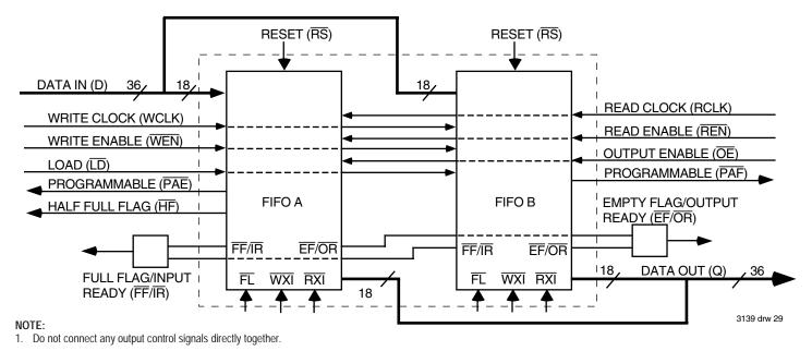
Figure 29. Block Diagram of the two FIFOs contained in one IDT72805LB/72815LB/72825LB/72835LB/72845LB configured for a 36-bit Width Expansion
