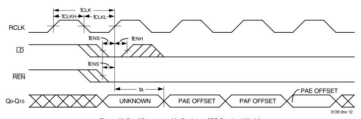
Figure 12. Read Programmable Registers (IDT Standard Mode)
