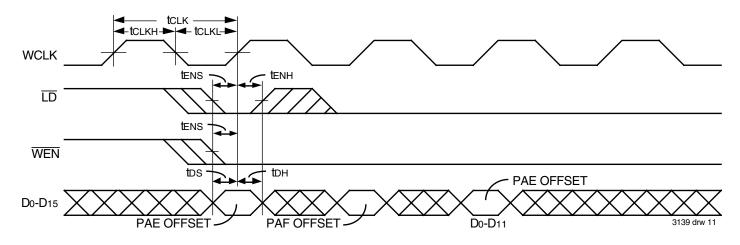
Figure 11. Write Programmable Registers (IDT Standard and FWFT Modes)
