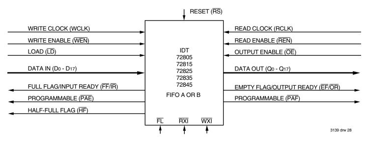
Figure 28. Block Diagram of Single 256 x 18, 512 x 18, 1,024 x 18, 2,048 x 18, 4,096 x 18 Synchronous FIFO (One of the two FIFOs contained in the IDT72805LB/72815LB/72825LB/72835LB/72845LB)
