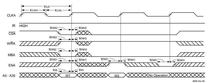
Figure 5. FIFO Write Cycle Timing
