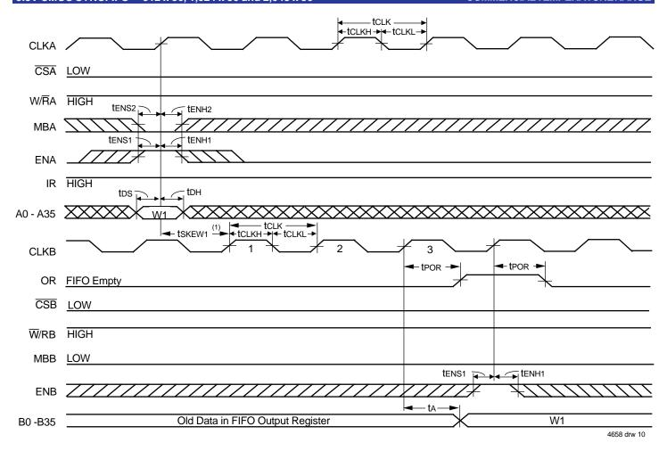
Figure 7. OR Flag Timing and First Data Word Fall Through when the FIFO is Empty
