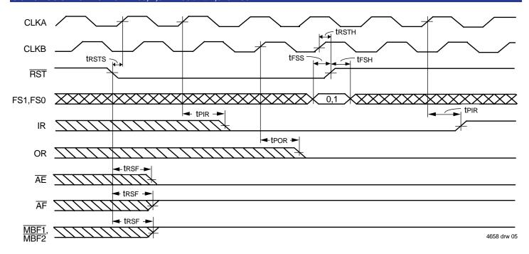
Figure 2. FIFO Reset and Loading X and Y with a Preset Value of Eight
