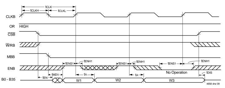
Figure 6. FIFO Read Cycle Timing
