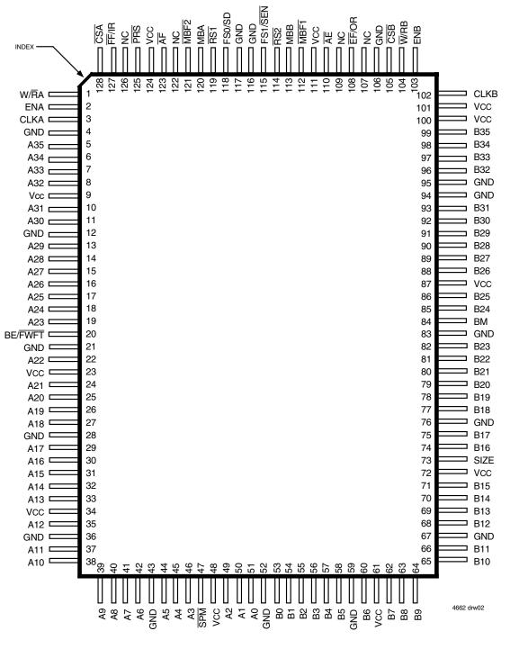
NOTE: 1. NC – no internal connection TQFP (PK128-1, order code: PF) TOP VIEW
