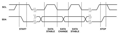
FIGURE 16. VALID DATA CHANGES, START AND STOP CONDITIONS
