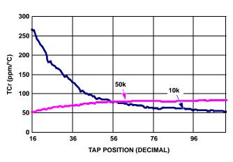
FIGURE 11. TC FOR RHEOSTAT MODE IN ppm
