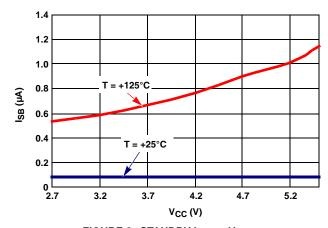
FIGURE 2. STANDBY  $I_{CC}$  vs  $V_{CC}$
