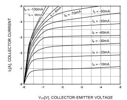
Figure 1. Static Characteristic
