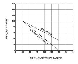
Figure 5. Derating Curve of Safe Operating Areas
