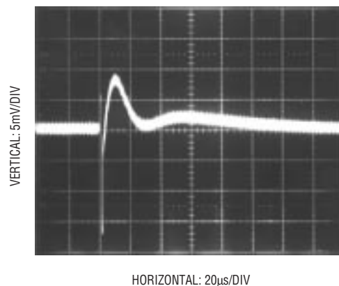
Figure 14. Poor Op Amp Settling Can Cause A/D Errors
