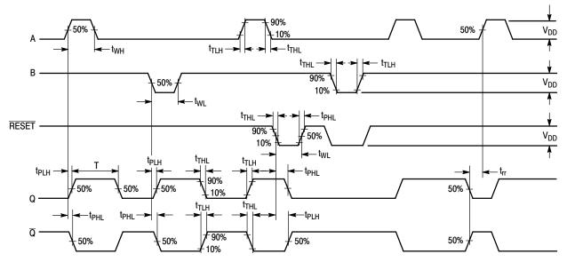
Figure 4. Switching Test Waveforms
