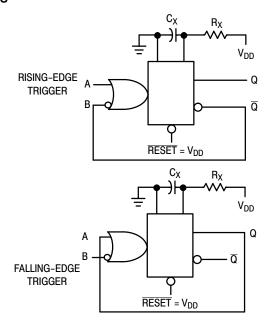
Figure 13. Non-Retriggerable Monostables Circuitry
