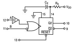
$R_X$  AND  $C_X$  ARE EXTERNAL COMPONENTS.  $V_{DD}$  = PIN 16  $V_{SS}$  = PIN 8, PIN 1, PIN 15
