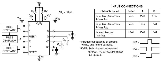
Figure 3. Switching Test Circuit
