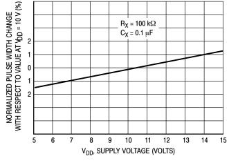
Figure 6. Typical Pulse Width Variation as a Function of Supply Voltage V<sub>DD</sub>
