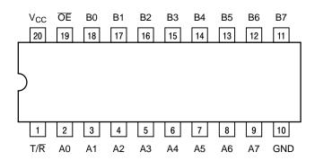
Figure 1. Pinout (Top View)
