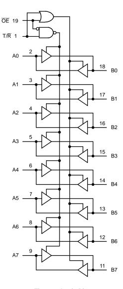
Figure 2. Logic Diagram
