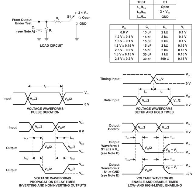
NOTES: A. C, includes probe and jig capacitance.
