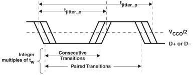
Figure 3. Output Jitter
