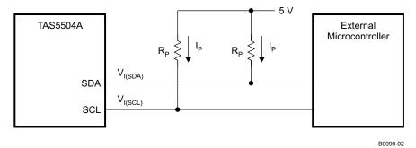
Figure 1. I<sup>2</sup>C Pullup Circuit (With No Series Resistor)
