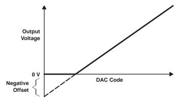
Figure 5. Effect of Negative Offset (Single Supply)
