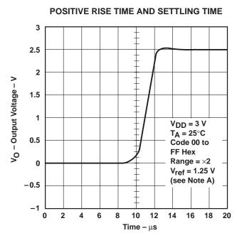
NOTE A: Rise time =  $2.05 \,\mu$ s, positive slew rate =  $0.96 \,V/\mu$ s, settling time =  $4.5 \,\mu$ s.
