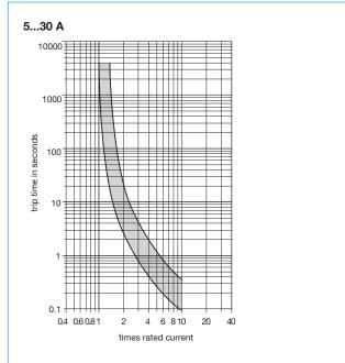
The time/current characteristic curve depends on the ambient temperature prevailing. In order to eliminate nuisance tripping, please multiply the circuit breaker current ratings by the derating factor shown below. See also section 9 – Technical information.
